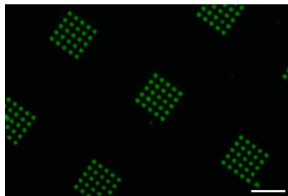
FIGURE 2. Immunofluorescent staining image of fibronectin coated on the patterned Ti-Au coated glass surface. Scale bar, 20 \mu\text{m} .
