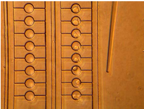
FIGURE 7. MLO-Y4 cells seeded into the microchambers using the micropipette transfer seeding technique.
